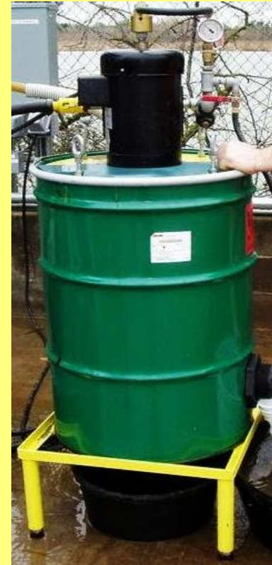
LEFT - Drum Version of iCON Concentrator showing the 45-gallon metal drum as an integral part of its structure. (photo: 'Rusty Happy Cam' of Alaska Gold Forum)
