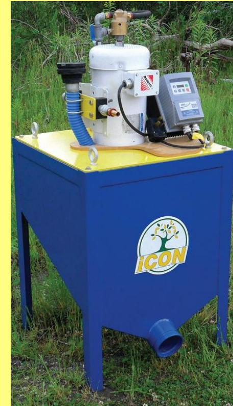
RIGHT - Current Version of iCON Concentrator, with the 45-gallon drum now discarded in favour of a simple box structure supported on four legs. (photo: www.iconcentrator.com )
